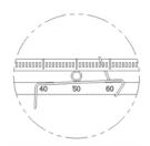
8. Check the valve stroke. The stroke marks are indicated on the feedback lever. Position the connection pin at the number on the feedback lever which corresponds to the desired valve stroke. To adjust, mover the bracket or the connection pin or both.
